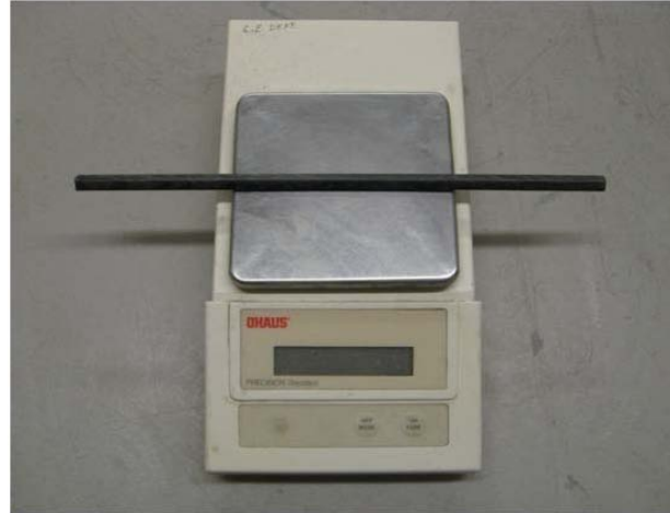
Figure 5-1. Measuring the weight of pultruded AS4 CFRE rod using an accurate scale ( \pm 0.01\text{g} )
